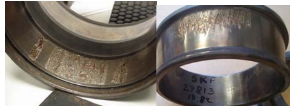
Cup and Cone Spalls – Package Bearing (PB)
