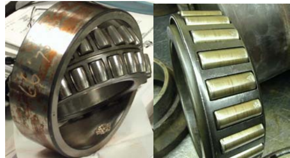
Cup Fault in Axle Box Roller Faults in PB
