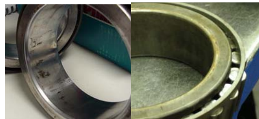
Fretting and Back Face Wear
